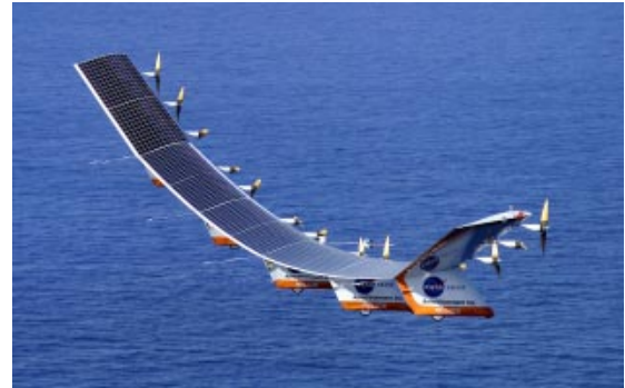
AeroVironment's solar-powered Helios Prototype flying wing on July 14, 2001, over the Pacific Ocean on its first test flight. The 18-hour flight from the U.S. Navy's Pacific Missile Range Facility, Kauai, Hawaii, was in preparation for the attempt to reach sustained flight at 100,000 feet altitude. On August 13, 2001, Helios flew to more than 96,500 feet, achieving status as the highest-flying nonrocket-powered aircraft in the world. The true airspeed was about 21 mph during take-off, reaching about 170 mph at peak altitude.
