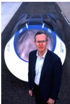
Paul MacCready and the solar-powered Sunraycer, AeroVironment's first land vehicle, built for GM and Hughes Aircraft. The goal was to advance transportation technology that makes fewer demands on Earth's resources and environment. The Sunraycer won a 1,867-mile race across Australia in November 1987, averaging 42.6 mph, 50 percent faster than the second-place vehicle. According to Engineering and Science magazine (Fall 1987), the Sunraycer scored the lowest drag coefficient ever recorded in Caltech's 10-foot wind tunnel.
